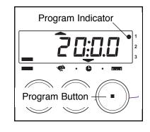
manual mode, press the program button until the program indicator disappears. The programs will be selected in the following order: program 1 (Interval), program 2 (Aerobic), program 3 (Fat Burn), manual mode.
